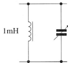
Which of the following tuning capacitors allows the radio to tune to carrier frequencies between 0.8MHz and 2.8MHz.
