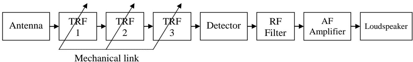
In the TRF radio receiver above there are three tuned RF amplifier circuits which amplify and select a particular carrier frequency. For any output to be heard from the loudspeaker all **three** tuned amplifier circuits must select exactly the same frequency, and hence the reason for the mechanical link between each of the three TRF stages. All three variable capacitors are mounted on the same shaft so that when one is altered the other two change to the same position at the same time.
