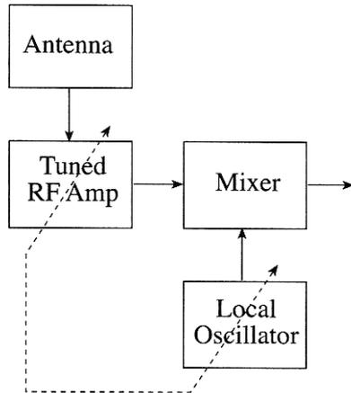
(a) The tuned RF amplifier has been tuned to a frequency of 1 MHz. The local oscillator output is measured at 1.45 MHz. What four frequency signals will be present at the output of the mixer.
