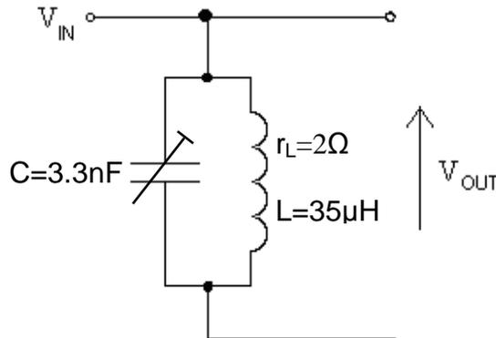
(a) Calculate the resonant frequency of the filter.
