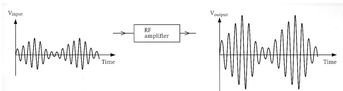
Now the RF signal will be much larger and it will be possible to select more stations than without the RF Amplifier. The radio has better sensitivity but has the same selectivity as the Simple Radio Receiver, because cross talk from adjacent radio stations is also amplified with the selected channel. The addition of an Audio Frequency Amplifier after the RF Filter will allow the output to be passed through to a loudspeaker, instead of headphones.
