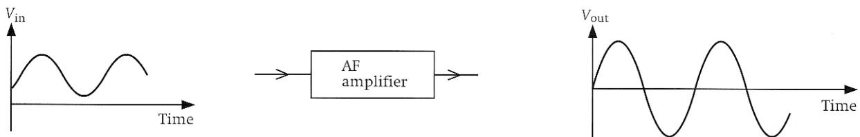
An AF amplifier is designed to enlarge signals at frequencies in the audio frequency range (20 to 20 kHz).
