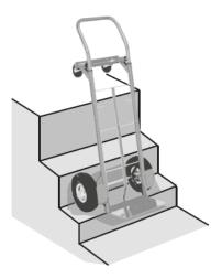
The wheels of the trolley always stay in contact with the steps on the way up.
