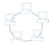
In a ring network, computer systems are connected in a ring or a loop. Packets are sent around the ring, being passed from one computer system to the next until they arrive at their destination.
