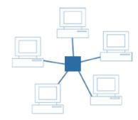
In a star network, each computer system is connected to a central node, also known as a hub.
