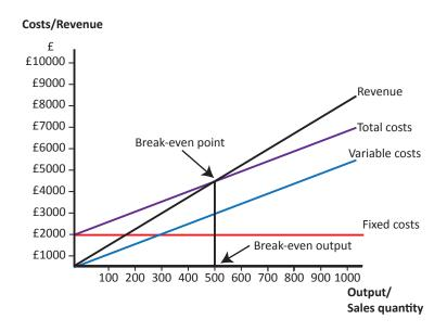
The point where the revenue line cuts the total costs line is break-even point. Draw a vertical line straight down from the break-even point; this will give you break-even output. A horizontal line drawn from break-even point to the costs/revenue axis will give you break-even costs/revenue.
