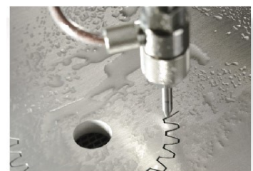
Water jet Cutting Steel
