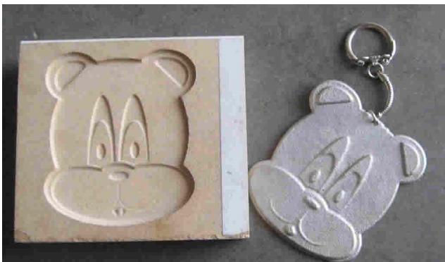
Mould created to cast Pewter
