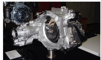
*Car Gear boxes bought in ready to be assembled on to the car*
