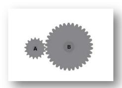
To decrease the speed of the output the driver gear is smaller than the driven gear.
