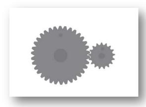
To increase the speed of the output the driver gear is larger than the driven gear.
