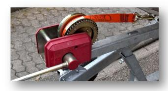
The radius of the driven gear is 4 times the radius of the driver.
