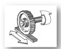
A DVD player also uses a rack and pinion to drive the disk tray in and out.
