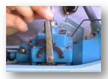
Ratchet and pawls are commonly used in lifting equipment to prevent the load falling once it has been lifted. These mechanisms can also be used to produce a regimented stepped rotational movement. Slippage of the ratchet is prevented by the spring. If the spring is pulled back sufficiently to disengage the pawl from the wheel, the load will fall.
