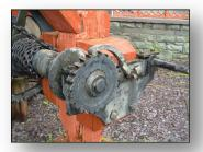
To allow the ratchet to be released the pawl is raised. A spring is usually used to keep the pawl in place against the ratchet.
