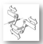
The saw blade on this mechanical hack saw moves forward and backwards in a reciprocating motion.
