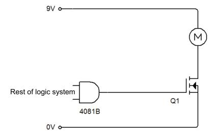
The motor is rated at 9 V, 8 A and the MOSFET has a value of  $g_{\rm M}$  = 1.6 S.
