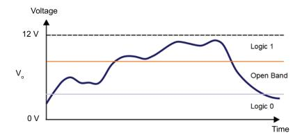
Logic gates require input signals that change rapidly between logic states. The analogue signal shown in the graph could remain in the open band for long periods of time, causing unpredictable behaviour and possible damage of a logic gate with which the sensor is interfaced.
