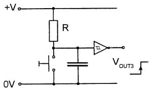
The value of capacitor used depends on how fast you want to count. A value in the range 1–10  $\mu$ F works well for most applications.
