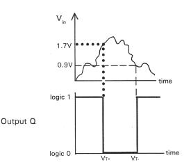
A **comparator** could be used to improve the rise time of a sensing sub-system but, as there is no deadband, minor changes in the signal from the sensor near the switching threshold could cause the comparator output to switch rapidly and repeatedly between logic 0 and 1.
