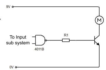
a) Calculate the value of R1 which will limit the base current to 5 mA.
