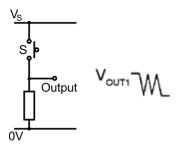
The graph below shows the results of switch bounce on the output of a switch unit:
