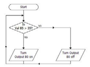
In the example above, if the Value of the analogue input that's connected to input B5 goes above 35 °C then some cooling fans connected to Output B0 are switched on. When the value of input B5 falls below 35 °C then the cooling fans are switched off.
