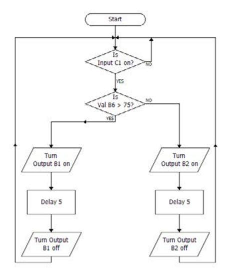
In this example, we have used a decision box to check if the doorbell switch has been pressed. If the switch is not pressed then it is continuously tested until it is. Only when the doorbell switch is pressed will the program continue past the first decision box. Then, if it is dark (B6>75) then LED is switched on, but if light (B6<75) then the buzzer is switched on.
