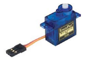
The servo motor is an assembly of four parts: a DC motor, a gear reduction unit, a potentiometer and a control circuit.
