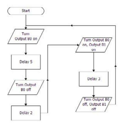
You should notice that when both LEDs have been turned off the program loops back to the first flowchart command so the program runs continuously. Also at the two points in the program where both LEDs are turned on or off this has been achieved with a single command in each case.
