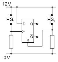
Pressing switch  $S_1$  sets the latch (Q = logic 1). Pressing switch  $S_2$  resets the latch (Q = logic 0).
