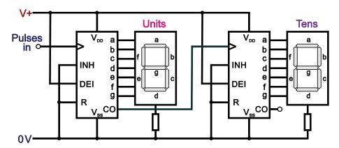
**Note:** The first of the circuits above has individual current-limiting resistors for each LED segment. In the bottom two circuits, the segments share a common current-limiting resistor. The disadvantage of this arrangement is that the current through each segment depends on how many segments are lit, causing slightly different levels of illumination for different numbers.
