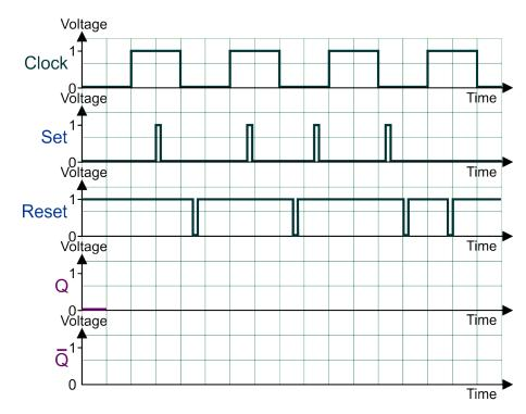
**3.** The graphs show the signals applied to the clock and data inputs of a rising-edge triggered D-type flip-flop.
