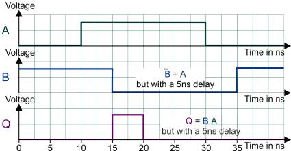
The result is that the transition gate generates a very short pulse of just 5 ns duration on the rising edge of the pulse on input  $\mathbf{A}$  – the edge triggering we were looking for!
