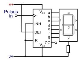
To link together a number of 4026 counters, the 'carry out' terminal on the first is connected to the clock input on the next.
