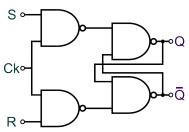
The NAND gates on the left send them a logic  $\mathbf{0}$  signal only when both of their inputs are logic  $\mathbf{1}$ . In other words, the  $\overline{\mathbf{Q}}$  and  $\mathbf{Q}$  outputs change only when:
