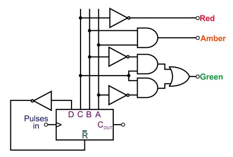
The counter resets as soon as output  ${\bf D}$  goes to logic  ${\bf 1}$ , i.e. on the eighth pulse. The sequence then repeats.
