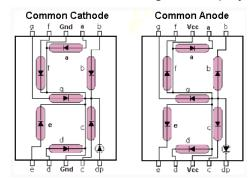
By lighting different combinations of LEDs, the decimal number set can be displayed. Here, a set of three displays shows the number '326'. To do this, appropriate logic signals are applied to segments 'a' to 'g'. To create the number '3' on a common-cathode display, the following combination of signals is sent to the display:
