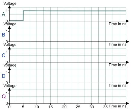
**2.** A transition gate is constructed from a NOT gate and a NAND gate. The propagation delay for each gate is 10 ns.
