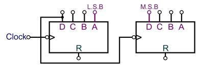
Propagation delay can be a problem, however, because earlier stages of the counter must change before the clock pulses reach the later stages. The more stages (bits) there are in the counter, the bigger the problem. Eventually, with high frequency clock pulses, changes in the most significant bits caused by one clock pulse may not be completed before the outputs of the least significant bits start to change as a result of the next clock pulse.
