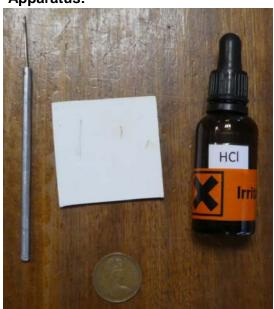
Mineral testing equipment: Streak plate/unglazed tile to test the colour of powdered minerals.
