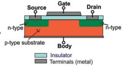
A MOSFET can be called a voltage-controlled device because the output current (from drain to source) is controlled by the voltage applied to the gate terminal. This controls the resistance of the conducting channel between the drain and the source, and hence controls the output current.
