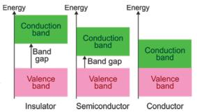
In insulators, there is a sizeable gap between the highest energy level in the valence band and the lowest level in the conduction band. This *energy band gap* means that an electron must gain considerable energy before it can take part in conduction. This is unlikely and so insulators do not conduct electricity very well. In other words, they have a high resistance to the flow of electricity.
