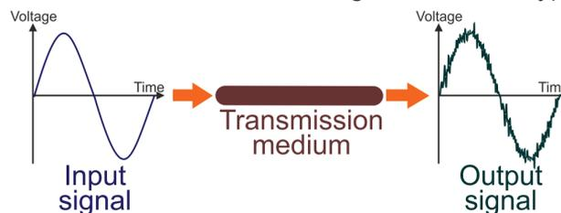
It is impossible to completely remove noise once it has been added to an analogue signal.
