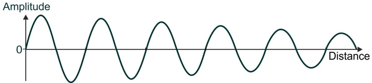
Attenuation can be thought of as a gain which is less than 1.
