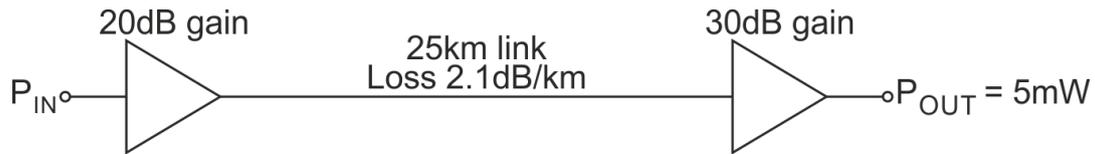
$$\text{Loss in link} = 25 \times -2.1 = -52.5 \text{ dB}$$
