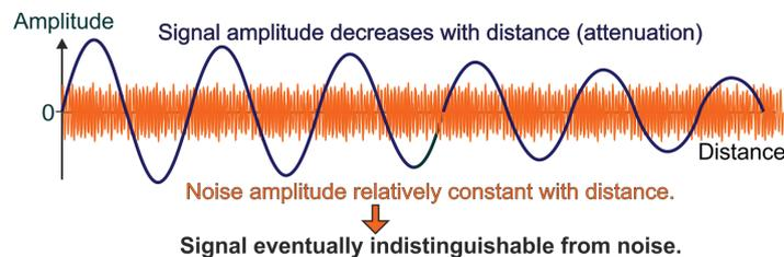
In the diagram, noise is not shown superimposed on the sinusoidal signal in order to show more clearly that the noise amplitude remains fairly constant while the signal amplitude decreases with distance.
